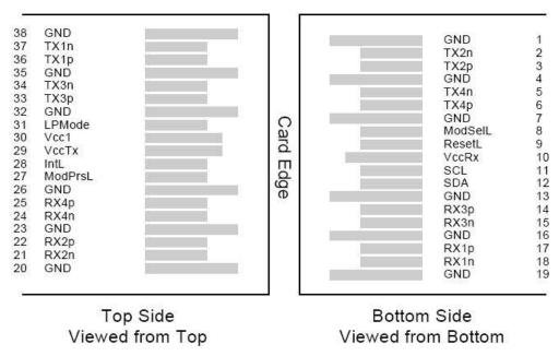
Figure 1. QSFP+ Transceiver Electrical Pad Layout
