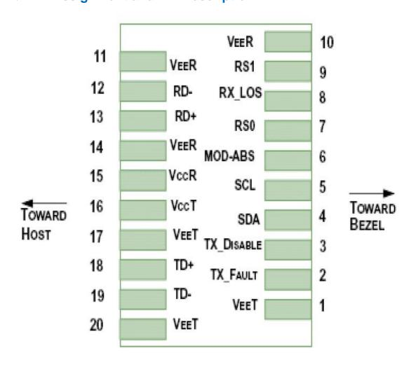
Figure 1. Diagram of host board connector block pin numbers and names
